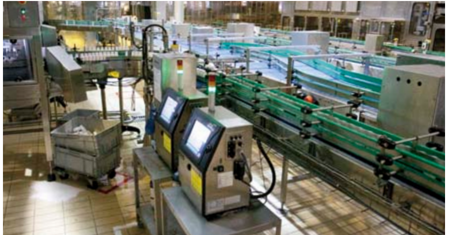
There are 40 units of the PXR-H450W models in 16 lines. Ingenuity has been employed by memorizing the print settings on each line in all of the Ink Jet Printers to enable swapping and repositioning the lines.
