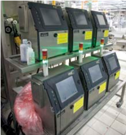
There are 40 units of the PXR-H450W models in 16 lines. Ingenuity has been employed by memorizing the print settings on each line in all of the Ink Jet Printers to enable swapping and repositioning the lines.
