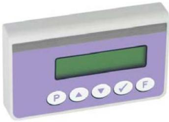
The optional OP2i keypad/display affords a single simplified interface for monitoring and control of the inverter/IPU-PSM system. It has a 2-line LCD display and keys that control its operation. The OP2i connects to the IPU-PSM “IEX2-OUT” connector by means of a standard RJ11 4-wire (telephone) cable. See [Figure 2-1](#).
