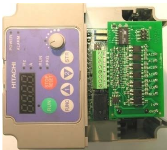
Figure 2-3, 115VIF-3 Correctly Installed in SJ200 Inverter
